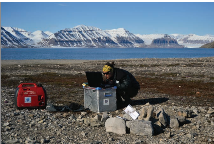
Figure 18 Setting up the thermistor string (Hassberg, June 2012)
