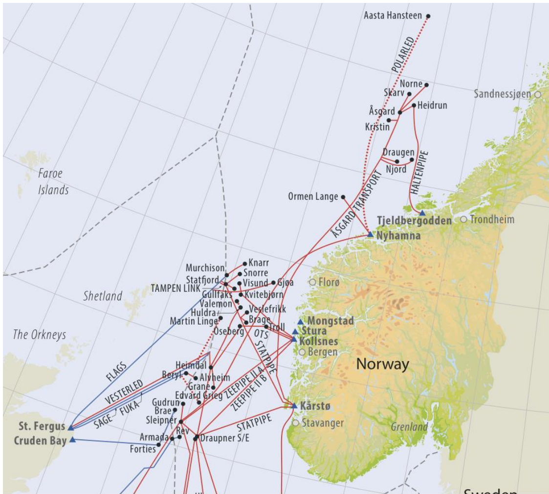
Figure 3.1 Map of the pipelines on the Norwegian shelf. The Polarled pipeline is denoted by the densely dotted line (Source: Norwegian Petroleum Directorate).
