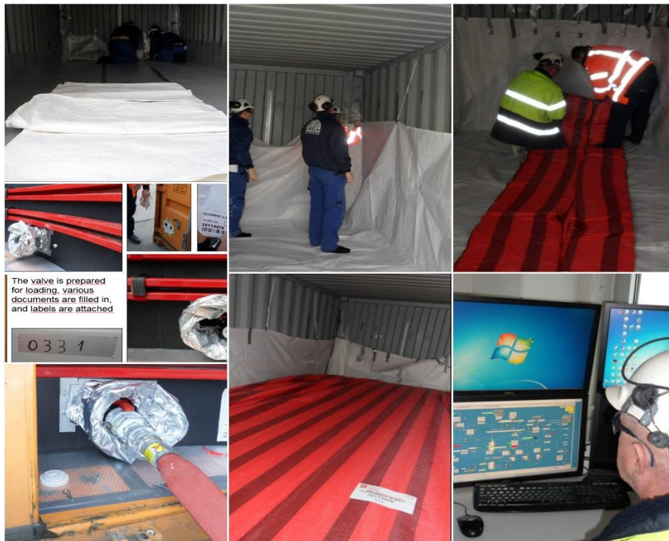
Figure 11: Preparation and loading of flexitank at Hustadmarmor (source: Vidar Hals)
