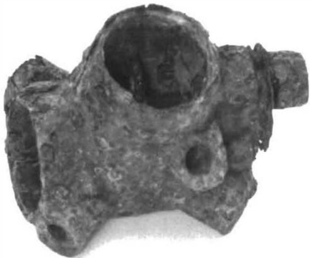
Fig. 54. Steel connecting casing from the Vaniman car found during the 1993 survey. The hole accommodated a one-inch pipe.
