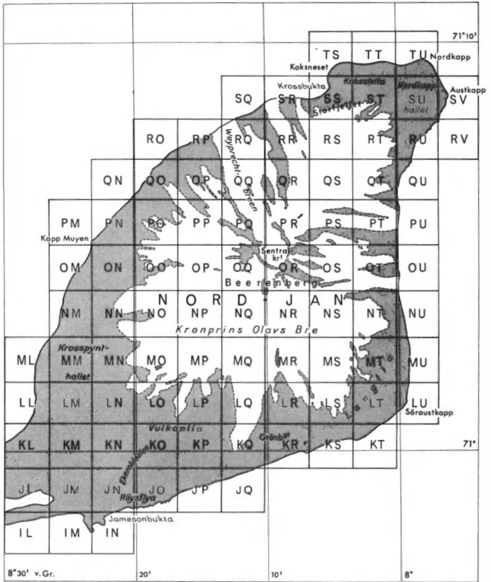
Fig. 2. Alphabetical key to 2 km square field mapping slips used by the Berenberg Expedition. Rock samples are located using a grid reference having its origin in the south-west corner of each slip.
