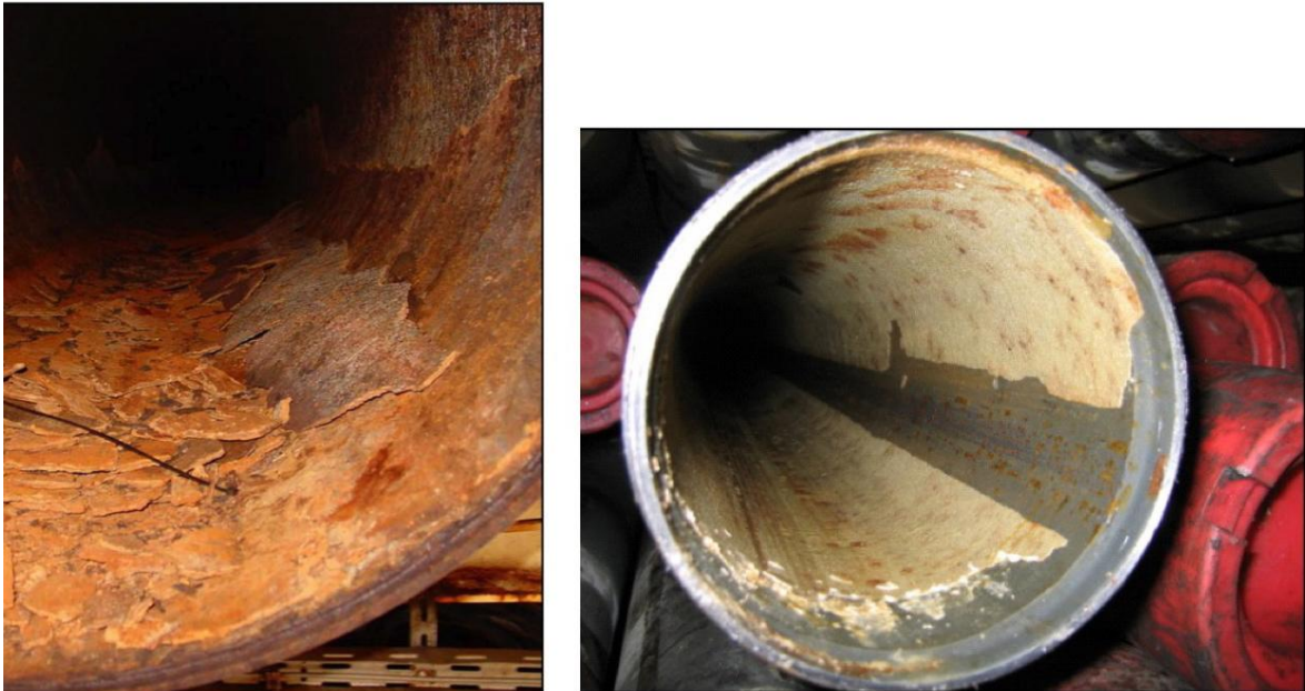
Figure 5: Scale formation inside pipes used for oil extraction (Varskog and Kvingedal 2009)
