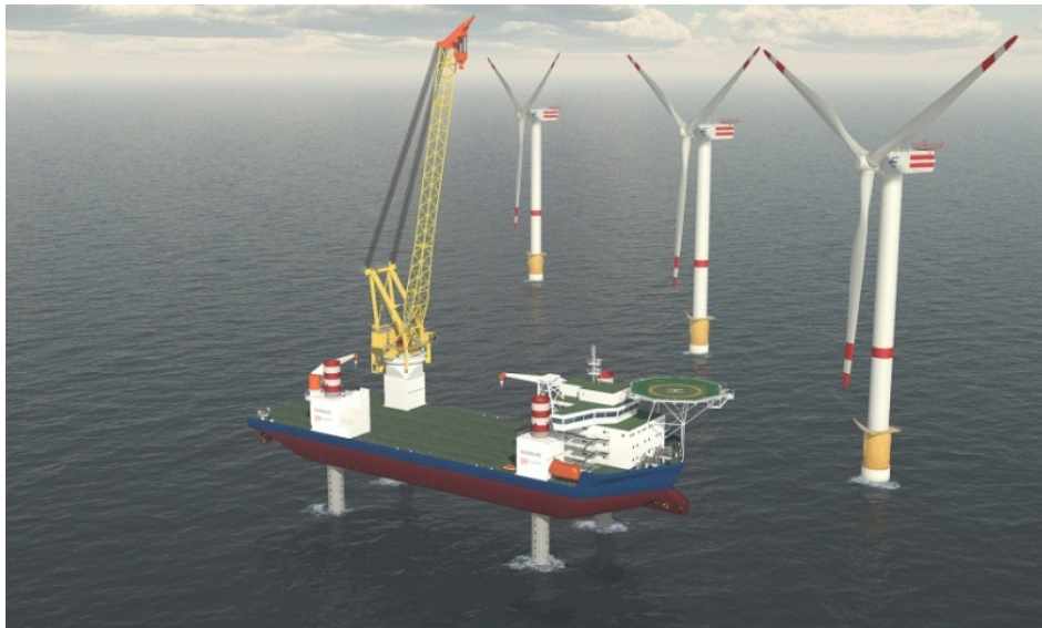
Figure 2.4 – Jack-up crane vessel during the installation phase [4]
