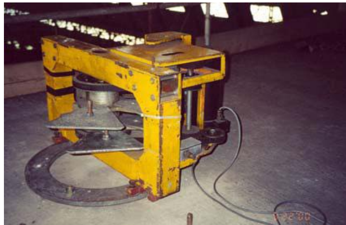
Figure 3.13. The vibration generator used by J.T. Snæbjörnsson et al. in 2000 [2].
