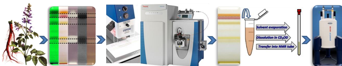
Figure 2. HPTLC-EDA-HRMS followed by preparative layer chromatography (PLC) isolation and NMR spectroscopy. 9
