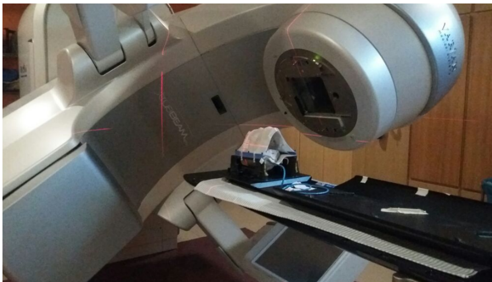
Figure 3. Irradiation set-up. Anthropomorphic 3D printed phantom positioned over the robotic couch of the Varian TrueBeam of the HIAE
