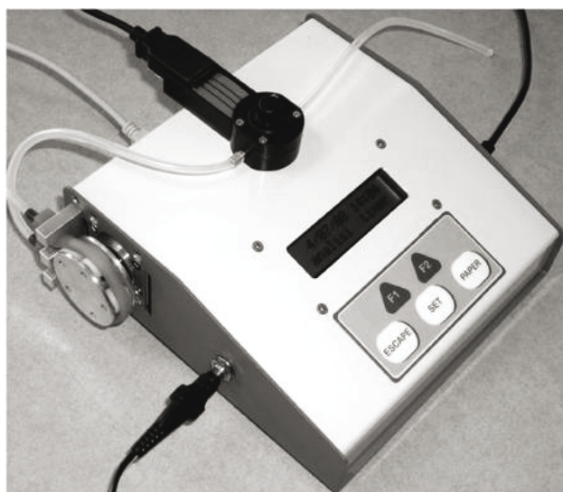
Fig.4. Photograph of the assembled bio-amperometer showing the flow cell with the electrode lodged in to perform the analysis.
