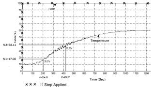
Figure 2.Temperature response for step applied (Output displayed in %).
