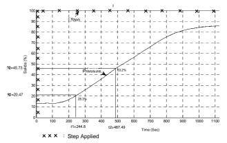
Figure 3.Pressure response for step applied (Output displayed in %).
