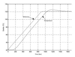
Figure 7.Temperature response applying Smith Predictor with PI by pole assignment method (Output displayed in  $\mathbb{C}$ ).
