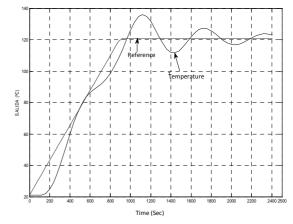
Figure 5.Temperature response applying controller PI by pole assignment method (Output displayed in  $\mathfrak{C}$ ).
