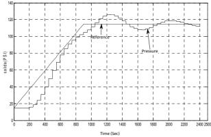
Figure 6.Pressure response applying controller PI by pole assignment method (Output displayed in PSI).
