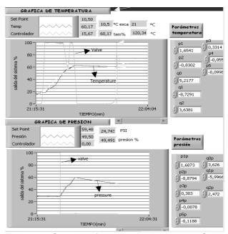
Figure 10. Control software main display type Smith Predictor for temperature and pressure variables (Output displayed in %).
