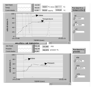
Figure 9. Control software main display type PI for temperature and pressure variables (Output displayed in %).
