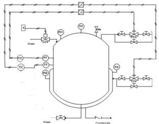
Figure 1.Autoclave instrumentation diagram.
