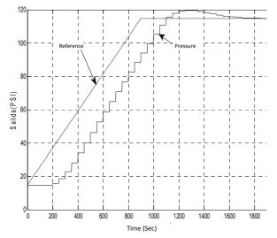
Figure 8.Pressure response applying Smith Predictor with PI by pole assignment method (Output displayed in PSI).
