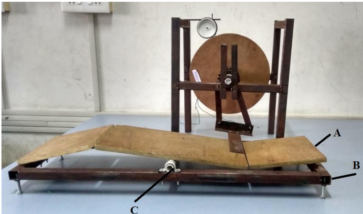
Fig. 3 Front view of the prototype model A as flat wood plate B as flat iron C as PVC pipe
