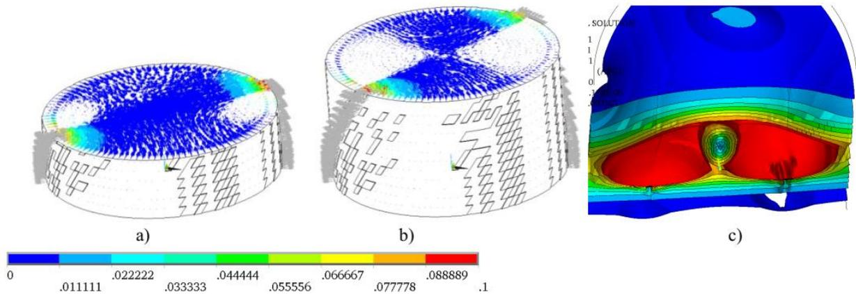
Fig. 7. The evaluation of the magnetic flux density vector  $B[T]$  in the modeled spiral arrangement of the permanent magnets, related to the volume of the cylinder: a) at one third of the cylinder height; b) at one half of the cylinder height; c) the magnetic flux density module  $B[T]$
