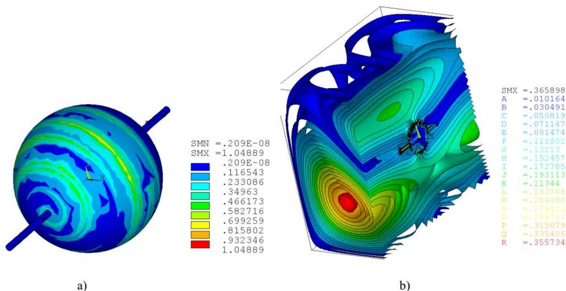
Fig. 8. The evaluation of the electric intensity  $E$  [V/m] in the modeled spiral arrangement of the wires, related to the volume for frequency  $f = 1$  GHz: a) at the sphere volume; b) around the spiral sphere volume
