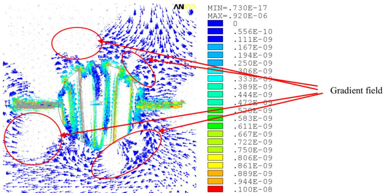
Fig. 9. The evaluation of the Poynting vector  $\Pi$  [W/m<sup>2</sup>],  $f = 1$  GHz in the modeled gradient spiral arrangement of the wires
