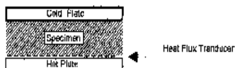
FIG. 1 Apparatus with One Heat Flux Transducer and One Specimen
