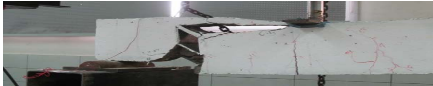
Figure 15: crack pattern for beam S-L-Steel
