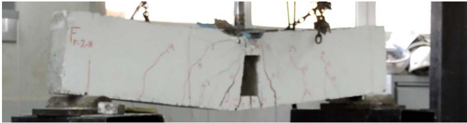
Figure 7: Crack pattern for beam F-R-2V
