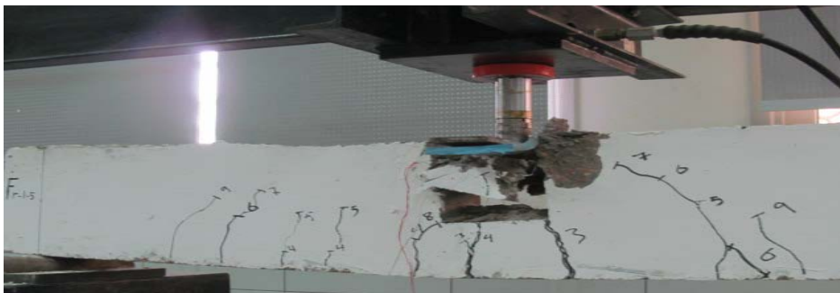
Figure 8: Crack pattern for beam F-R-1.5H
