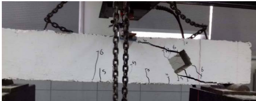
Figure 10: Crack pattern for beam S-S-45
