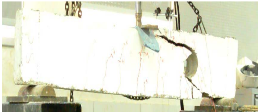
Figure 12: crack pattern for beam S-C
