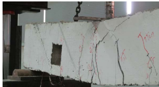
Figure 19: Crack pattern for beam S-R-N
