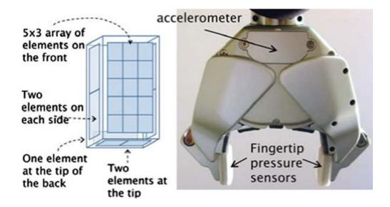
**Figure 4:** the PR2 robot gripper. The pressure sensors are attached to the robot's fingertips under the silicone rubber coating [2].
