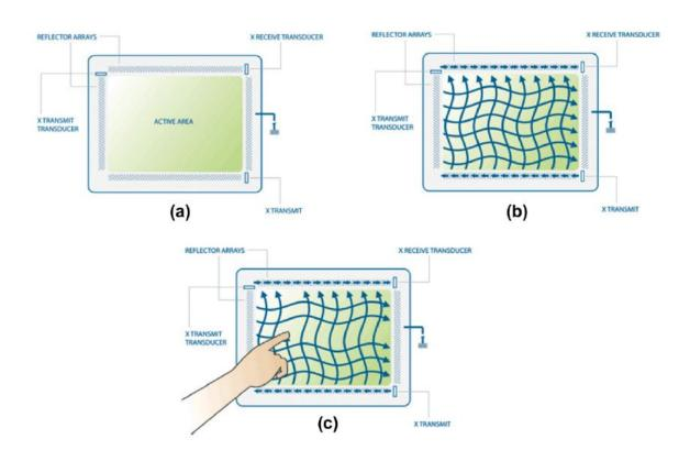
Figure 1: Surface acoustic wave touch screen (a). Constitution (b). Non-disturbed acoustic waves pattern, (c) Acoustic wave pattern when touched [2].
