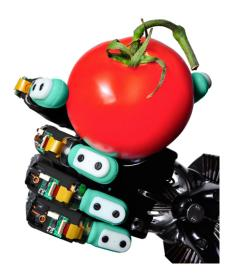
Figure 5: SynTouch BioTac tactile sensor [2].
