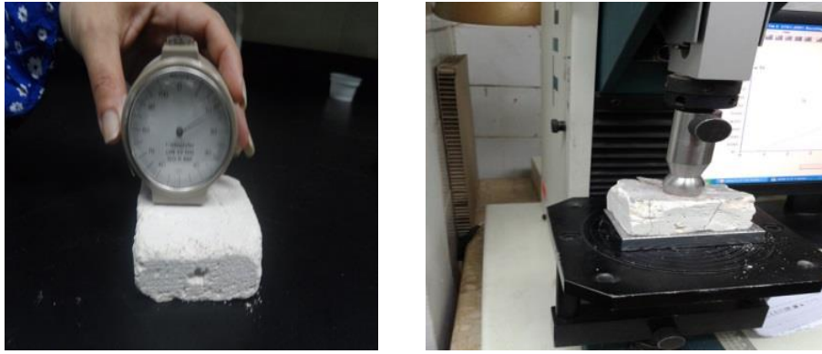
Figure 6: Testing samples for Hardness using Shore D and bursting strength test using Tinuis Olsen
