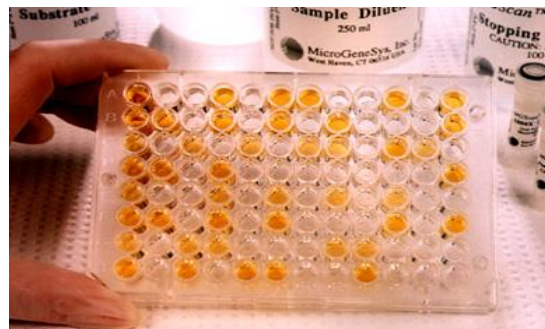
Figure 5: Microplate ELISA: coloured wells indicate reactivity. The darker the colour, the higher the reactivity
