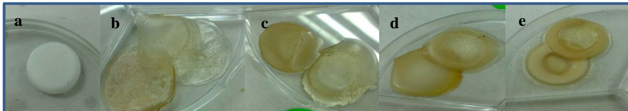
Figure 1: Composite Solid Polymer Membranes (a) White elastic gel membrane before dried (b) 4M MSA (c) 5M MSA (d) 6M MSA (e) 7M MSA
