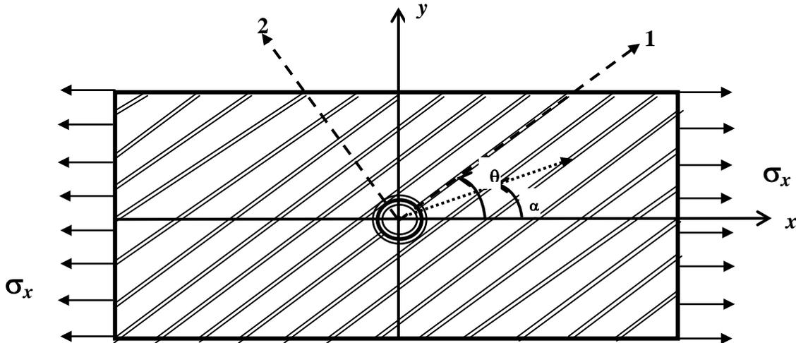
Figure 3: Composite plate with central hole subjected to uniaxial loading
