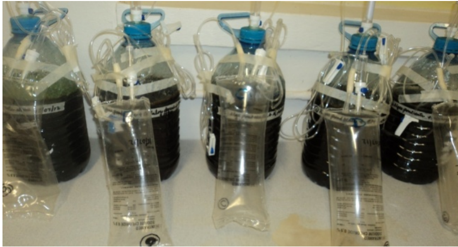
Figure 1. Simulated lab scale plastic anaerobic digester set and biogas production with various treatments: Control, C, C+N 1 , C+N 2 and C+N 1 +N 2 .
