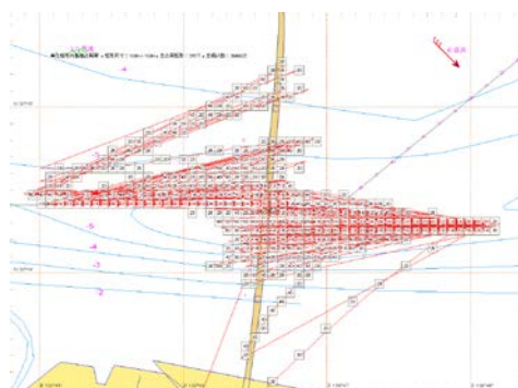
Fig. 4. The probability distribution of ship passing through Jiashao Bridge
