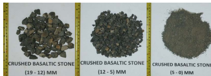
Plate1:Three Different Sizes of Crushed Basaltic Stone Product from Jebel Touryia
