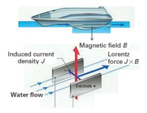
Fig. 1. Magneto-hydrodynamic propulsion principle
