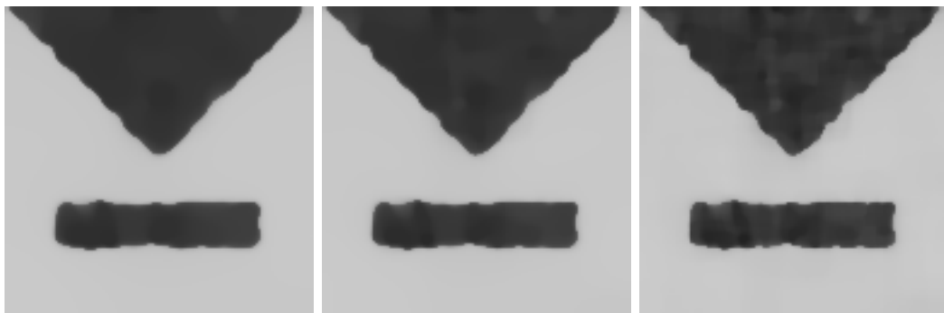
Figure 4.7: Influence of parameter \tau on the moment preserving diffusion, AOS scheme with Charbonnier diffusivity, p = 3, s = 127.5, \sigma = 0.0, \lambda = 0.05 ; Left: \tau = 5.0 , 100 iterations; Middle: \tau = 20.0 , 25 iterations; Right: \tau = 50.0 , 10 iterations.
