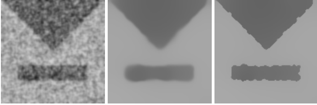
Figure 4.2: Noisy image filtered with different diffusivity functions; Left: Linear diffusion, implicit scheme, \tau = 0.1 , 10 iterations; Middle: Nonlinear isotropic diffusion, AOS scheme with Charbonnier diffusivity, \tau = 5.0, \sigma = 0.0, \lambda = 0.25 , 100 iterations; Right: Nonlinear isotropic diffusion, AOS scheme with Perona-Malik diffusivity, \tau = 5.0, \sigma = 0.0, \lambda = 2.0 , 100 iterations.
