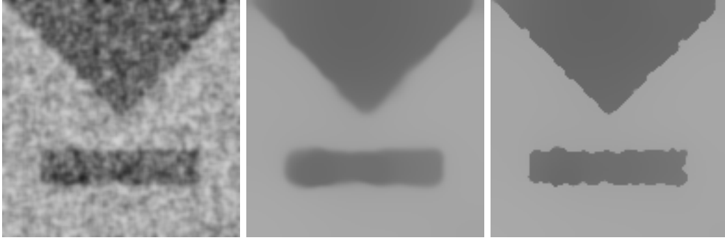
Figure 4.9: Noisy image filtered with different diffusivity functions; Left: Linear diffusion, implicit scheme, \tau = 0.1 , 10 iterations; Middle: Nonlinear isotropic diffusion, AOS scheme with Charbonnier diffusivity, \tau = 5.0, \sigma = 0.0, \lambda = 0.25 , 100 iterations; Right: Nonlinear isotropic diffusion, AOS scheme with Perona-Malik diffusivity, \tau = 5.0, \sigma = 0.0, \lambda = 2.0 , 100 iterations.
