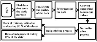
Figure 1. Block diagram of the chronological steps to process the data. Data preparation begins with finding the data that serves the study purpose, and ends with splitting the data into the training-testing-validation dataset and hold-out dataset.
