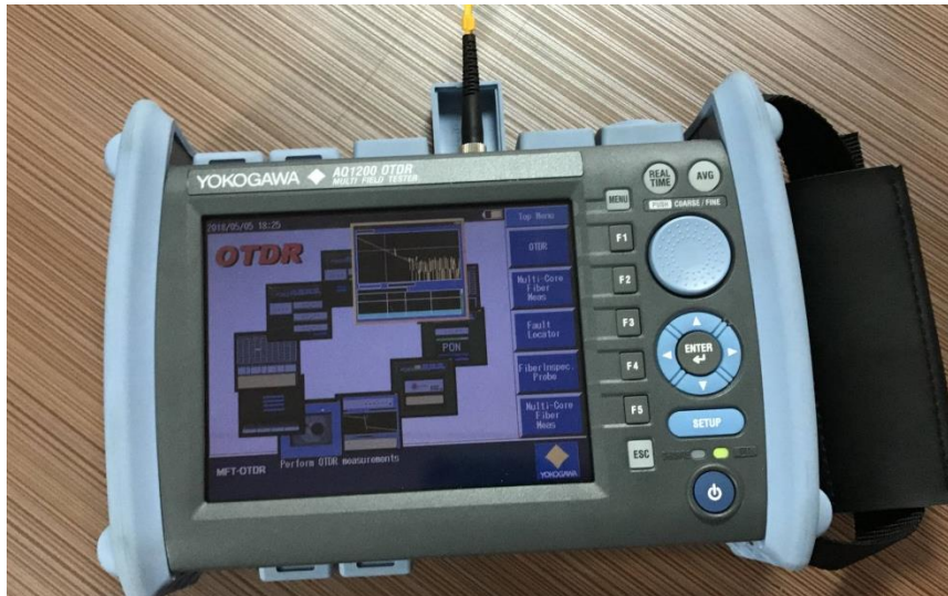
Figure 5. Optical mini-reflectometer YOKOGAWA.
