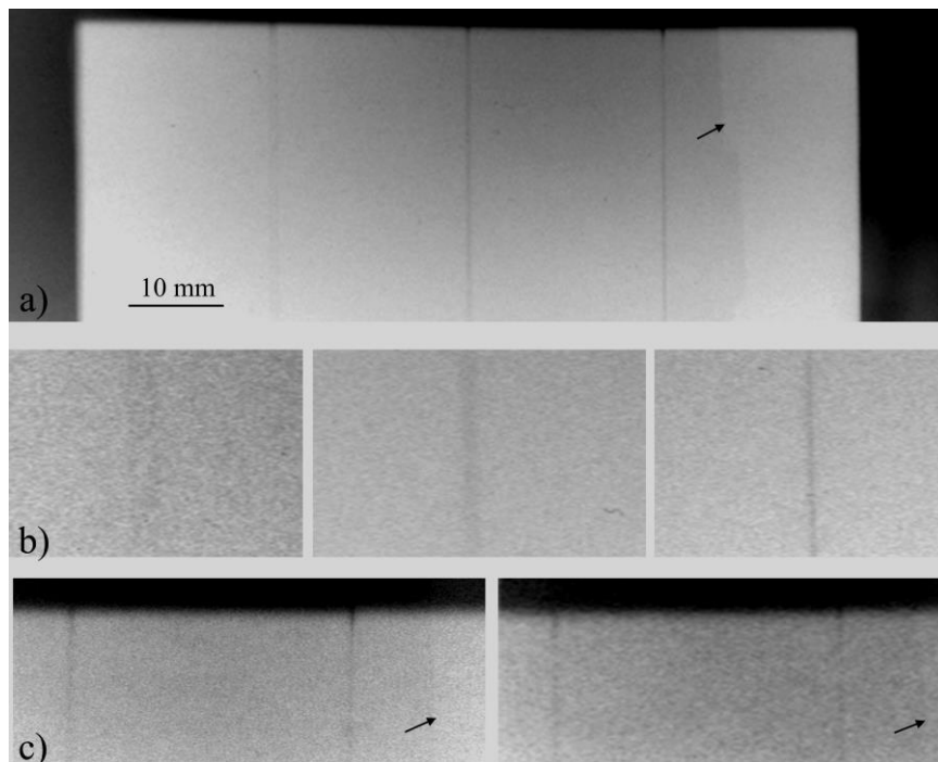
Figure 3. Images of the sample with 10 \mu\text{m} gaps between the steel blocks: a) the image obtained with magnification of 2.4; b) additional enlarged images of the left, middle and right gaps of the steel sample; c) images of the middle and right gaps in the upper part of the steel sample obtained with an additional steel plate-absorber with thickness of 20 (left) and 40 mm (right), respectively.
