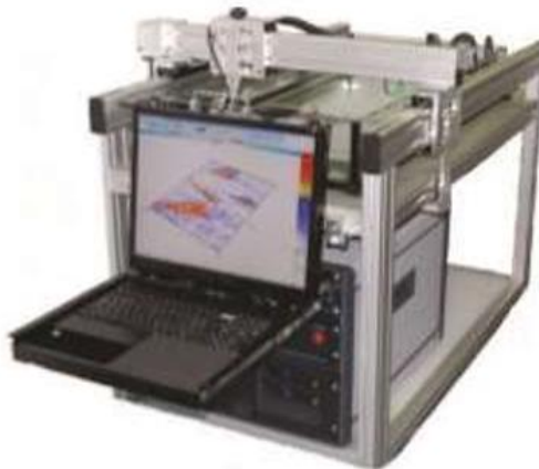
Figure 2. Ultrasonic tomography system IDEalSystem3D.
