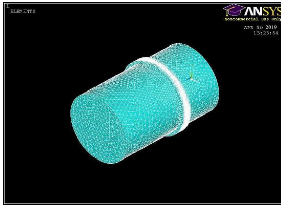
Figure 3 – Finite element model of the Nutation Speed Reducer
