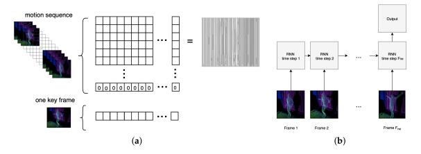
**Figure 6.** (a) The process of using a Convolutional Neural Network (CNN) for gestures-based emotion recognition shows the process of creating an matrices based on motion sequence. (b) The process of using a Recurrent Neural Network (RNN) for motion sequence analysis—each time step of the motion sequence is evaluated by a RNN.
