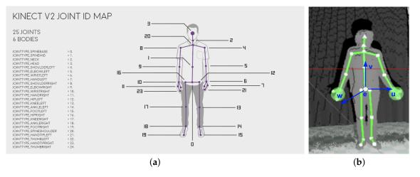
Figure 3. (a) Skeleton mapping in relation to the human body [33]. (b) An example frame of Kinect recording showing the skeleton.
