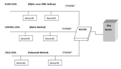
Figure 8. Test setup of industrial automation network with key establishment schemes.
