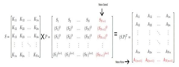
Figure 5. Device addition operation.
