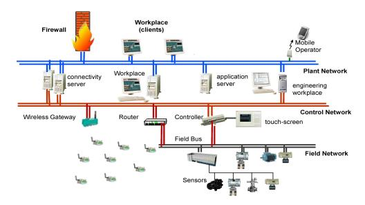
Figure 1. Industrial automation and control systems.
