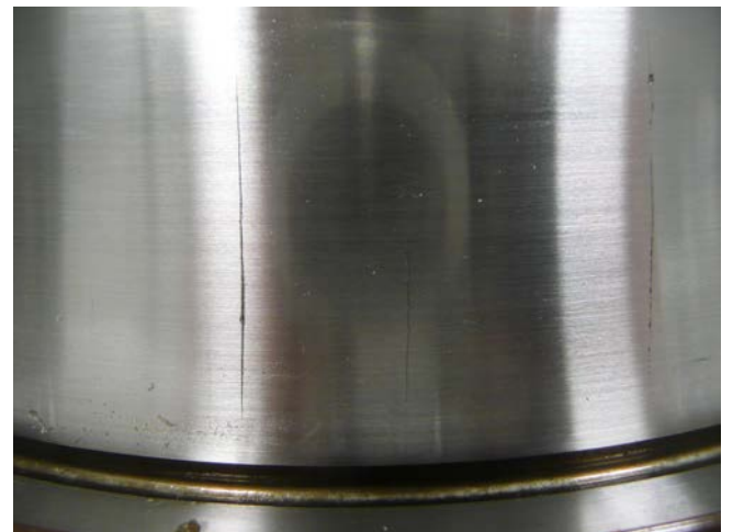
Figure 6: Axial crack on the inner ring of a bearing from service
