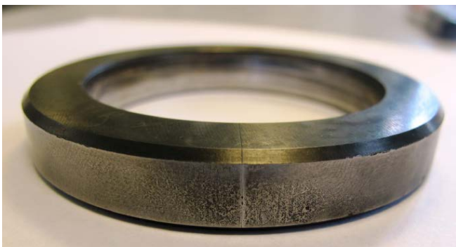
Figure 3 : Axial crack on ring B1.
