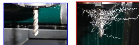
(a) Without chip (tap covered with Ni/cBN film) (b) With chip (tap covered with TiCN film) Fig. 2 Snap shot of tapping tool after
