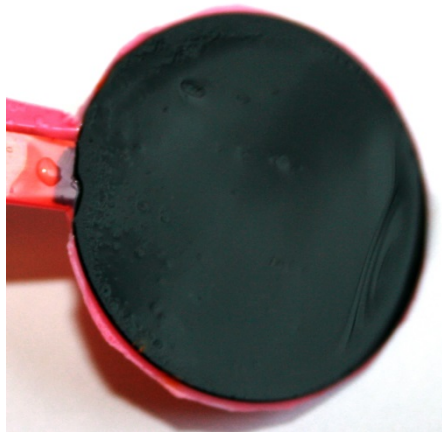
Fig. 36: The as-plated platinum black surface.
