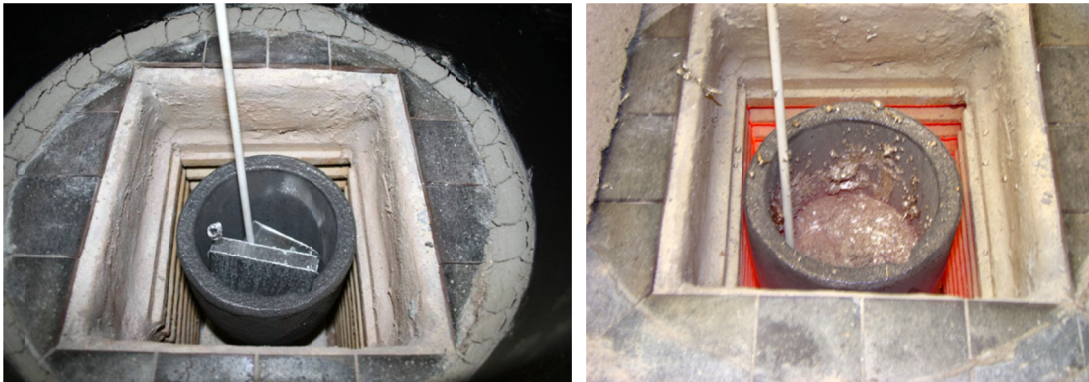
Fig. 44: The clay crucible used for the hot dip aluminising as placed in the furnace before and after melting of the aluminium.
