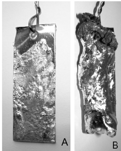
Fig. 45: Two hot dip aluminized nickel coupons. A) Without purging of argon gas and B) with purging of argon gas.
