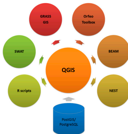
Figure 1. Open-source software packages integrated as part of the Water Observation and Information System (WOIS).
