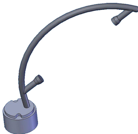
Figure 1. A 1D sonic sensor normally mounted from the inside of the spinner.
