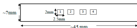
Fig. 1. Sketch of the sample, top side exposed into the finwalls between two tubes at furnace walls area. 4 different areas on the middle of each specimen were analysed under SEM/EDS.
