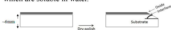
Fig. 2. Schematic view of the samples before and after polishing, the angle shown at the right figure was between 30° and 45°.
