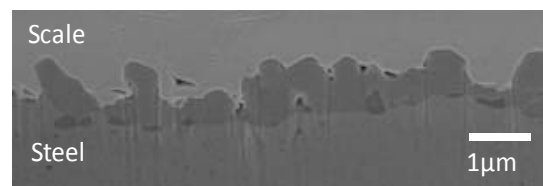
Fig. 6 SEM image of scale/steel interface when axial compression of 12.7 MPa is applied on during scale merging.
