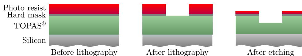
Figure 5.10: Etching of TOPAS ® was done without removing the resist from the hard mask. The hard mask was used to ensure masking even if the photo resist was completely removed. The hard mask material were either aluminum or silicon.
