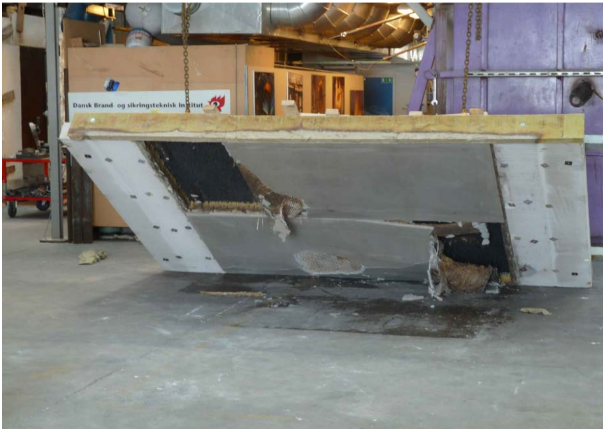
Figure 20: A failed fire test of a HPC sandwich panel tested at Dansk Brand- og sikringsteknisk Institut (DBI)
