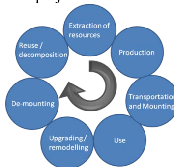
Figure 4: The life cycle of a building as met in the case project
