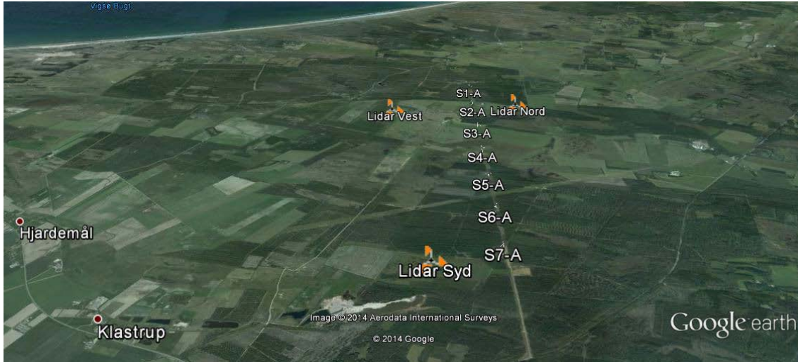
Figure 9: Google Earth image of seven test stand positions and three wind lidars
