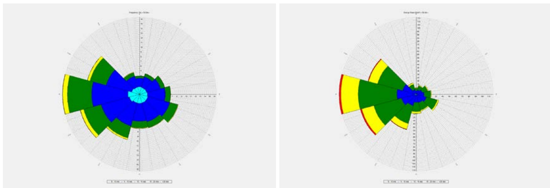
Figure 8: Wind direction frequency (left) and power density (right) distributions of MERRA long-term reference data at 50 m AGL
