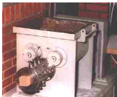
Figure A.2: Mechanical extruder used for large scale extrusions at CSIC in Madrid.
