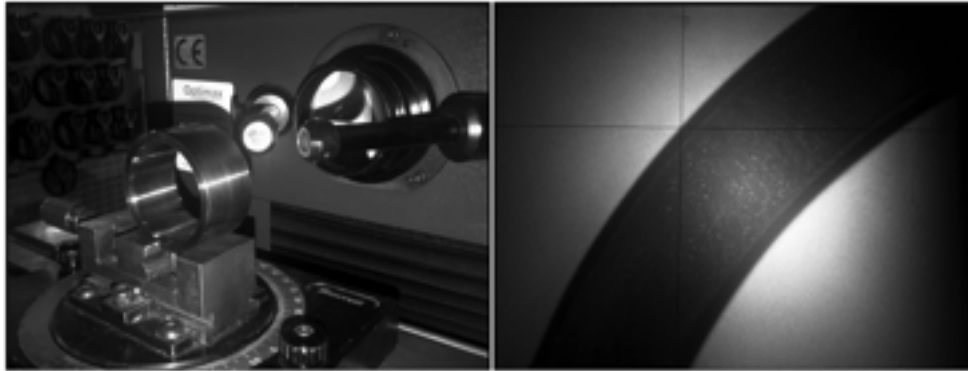
Figure 7. Optical comparator with bearing outer race in-situ, showing; lens and lights directed at the part mounted on the 4-axis table (left), and shadow-view of the bearing outer race (right)
