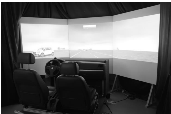
Fig. 1. Driving simulator cabin and projection planes.
