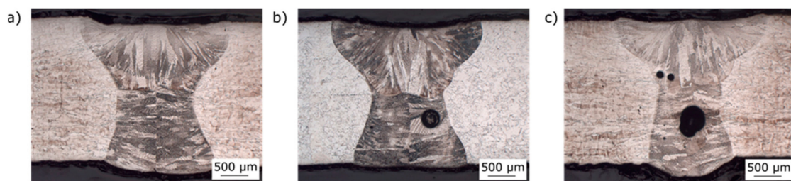
Figure 13. Cross sections of SLM-manufactured tubes of IN625 (overlap area): (a) IN625_WOHT_SLME, (b) IN625_HT_SLME, and (c) IN625_WOHT_SLME.
