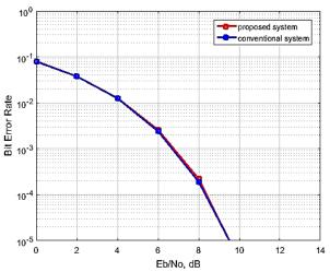
Fig. 8. BER performance comparison over AWGN channel
