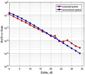
Fig. 9. BER performance comparison over flat fading channel
