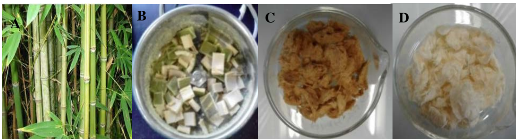
Figure 1: Photographs of A: the Tacuara Cane, B: pieces of cane cut untreated, C: delignified cane pulp, and D: bleached pulps
