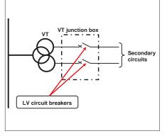
Figure 8. Voltage transformer junction box
