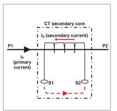
Figure 9. Current transformer connection
