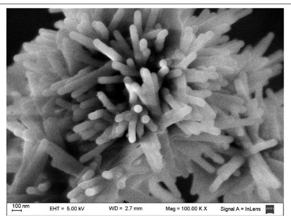
Figure 3: Silica precipitated from Na,SiO<sub>3</sub> at pH 12. Final Si(IV) concentration = 0.0065M.
