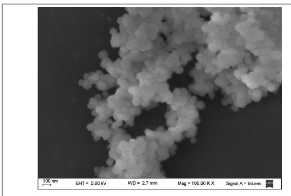
**Figure 5:** Silica precipitated from Na,SiO<sub>3</sub> at pH 9. Final Si(IV) concentration = 0.005M.
