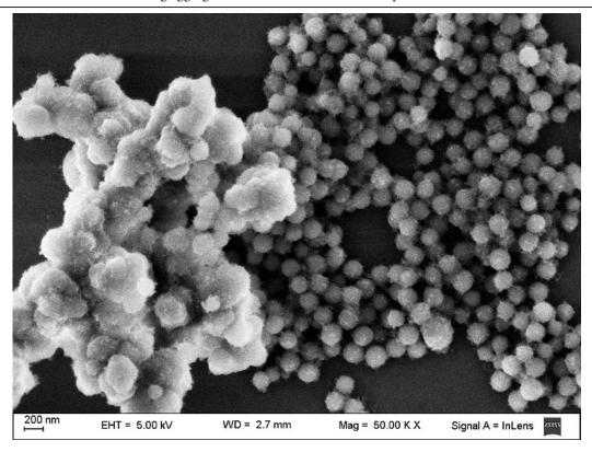
Figure 4: Silica precipitated from Na<sub>2</sub>SiO<sub>3</sub> at pH 8. Final Si(IV) concentration = 0.0065M.
