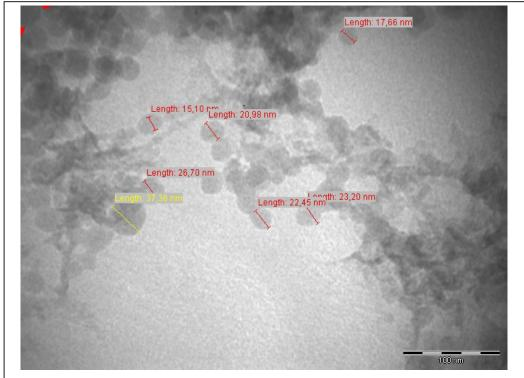
**Figure 8:** TEM micrographs of PFD containing silica nanoparticles. Note the homogeneous size and small diameter obtained.
